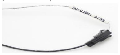
(2). TO ENTER SELF LEARN MODE, YOU WILL NEED TO CONNECT THE TWO WHITE WIRES FOR 5 SECONDS, THEN DISCONNECT, SELF LEARN WILL PAIR THE MOTOR TO THE CONTROLLER.
